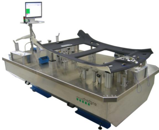
Test station - passenger car roof-liner
