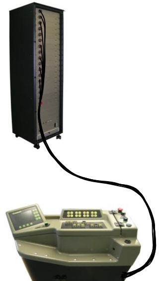
Test system for checking a control and monitoring console
